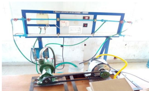
Fig3.3 Double pipe Heat Exchanger apparatus
